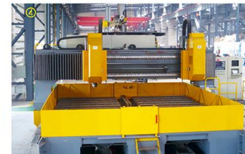
④ 龙门移动式数控平面钻床 Longmen Moving CNC Plane Drilling Machine
