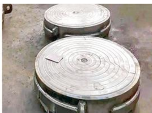
管板带极自动堆焊 Automatic strip welding of tube sheet
