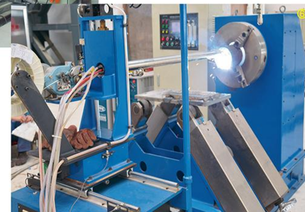
小直径内壁堆焊机 Overlay Welding Machine for Small Diameter Inner Wall
