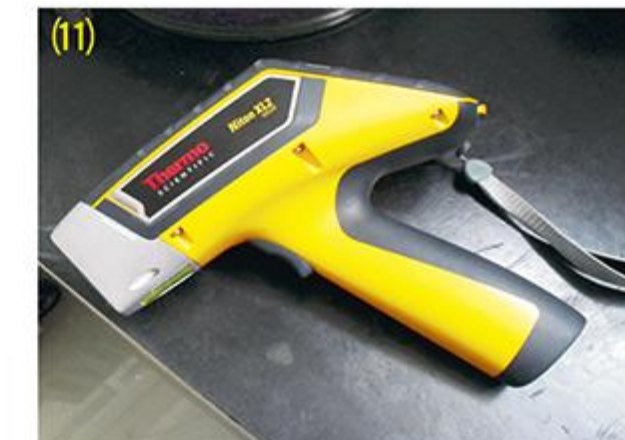
手持式合金分析仪 Therom Scientific Niton Handheld XRF All oy Analyzers
