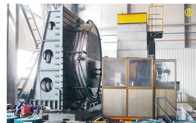
卧式双主轴数控深孔钻床 Horizontal & Biaxial CNC Deep-hole Drilling Machine
