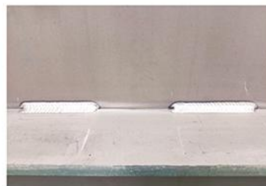
钛材等离子角缝焊接 Titanium Plasma Corner Welding
